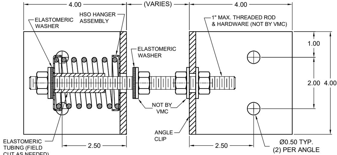
**EXTERNAL SPRING BRACKET INSTALLATION**
